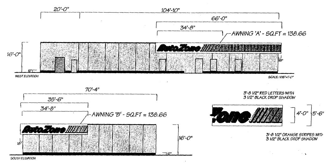
AWNING TO BE FABRICATED FROM 1" SQ. ALUMINUM TUBE WITH STRETCHED WHITE COOLEYBRITE #0606 FABRIC FACES. ILLUMINATE WITH TWO (2) ROWS OF EIGHT (8) 96" CWHO FLUORESCENT LAMP FIXTURES ON WEST ELEVATION AND TWO (2) ROWS OF FOUR (4) 96" CWHO FLUORESCENT LAMP FIXTURES ON SOUTH ELEVATION. MOUNT FIXTURES END TO END ON AWNING AT 24" ON CENTER.
