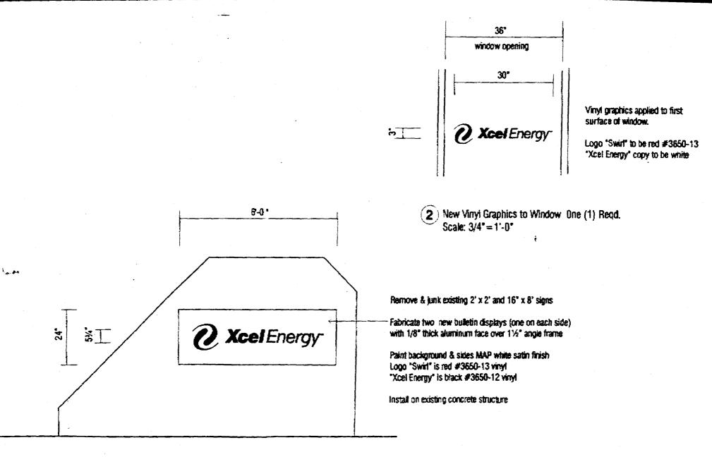
(1) New Signs to Existing Concrete Display Two (2) Required Scale: 1/2\*=1'-0\* Mar Ar ar
