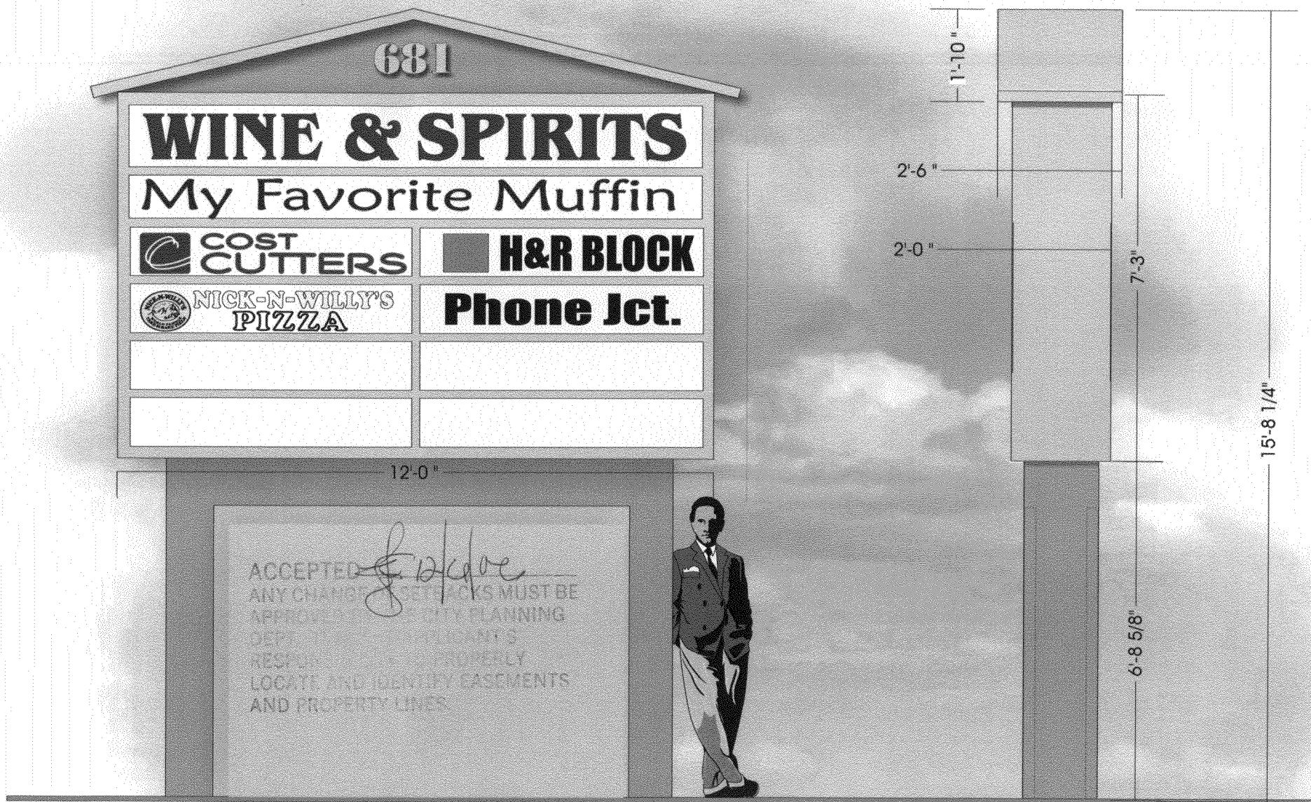
Double Face Internally Illuminated Sign Cabinet
