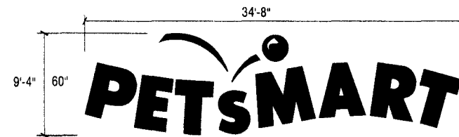
EXISTING "OLD STYLE" PAN CHANNEL LETTER SCALE: 1/8"=1'-0" 263.40 SQ. FEET
