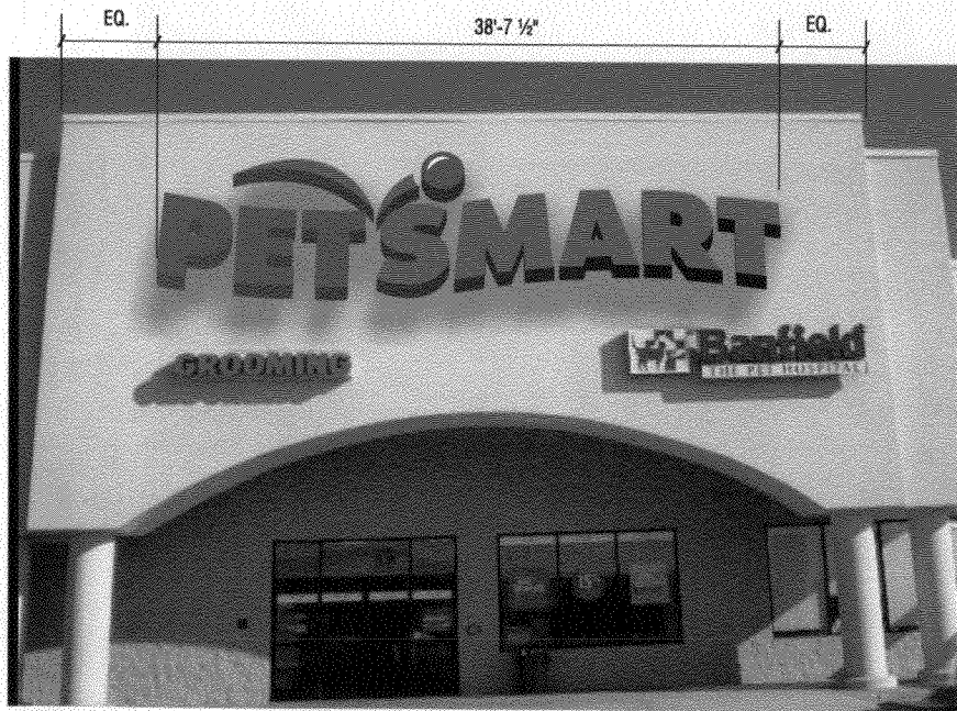
MFG. & INSTALL NEW 60" PETSMA RT CHANNEL LETTERS
