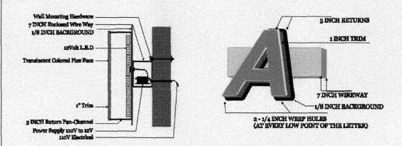
SPECIFICATIONS: Manufactured pan channel letters Faces: 3/16" orange plexiglass Trimcap: 1" gold Sidewalls: bronze Lighting: red LED Raceway: painted to match building Square Feet: 30 SQFT Final electrical 110V hook-up is to be done by a licensed electrician.
