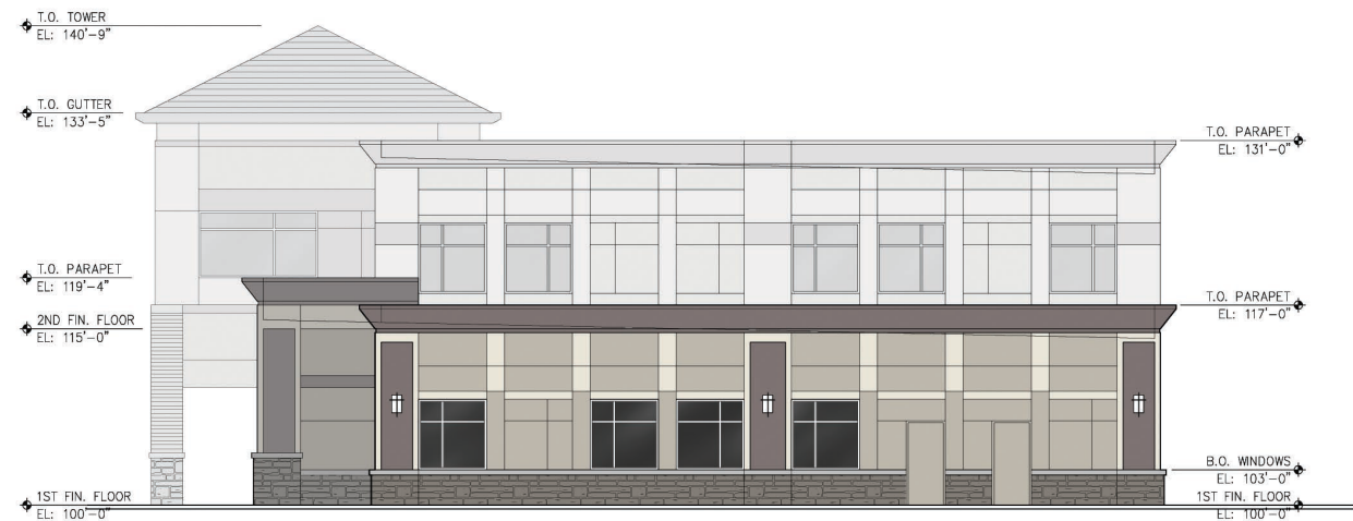
4 NORTH-WEST ELEVATION A3.1 1/8" = 1'-0"
