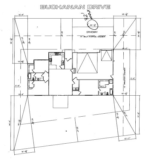
NOTE: DIMENSION LINES ARE PULLED FROM EDGE OF BRICK LEDGE. IF NO BRICK LEDGE EXISTS, DIMENSIONS WILL BE FROM EDGE OF FOUNDATION.
