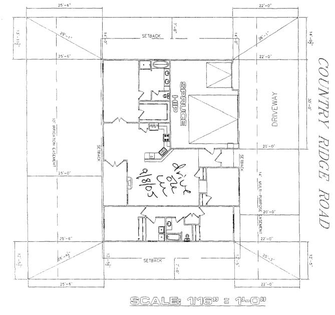
NOTE: GRADE MUST SLOPE AWAY FROM HOUSE 6" OF FALL IN THE FIRST 10' OF DISTANCE PER LOCAL BUILDING CODE. NOTE:: DIMENSION LINES ARE PULLED FROM EDGE OF BRICK LEDGE. IF NO BRICK LEDGE EXISTS, DIMENSIONS WILL BE FROM EDGE OF FOUNDATION. SITE PLAN INFORMATION SUBDIVISION NAME COUNTRY RIDGE ESTATES FILING NUMBER 1 LOT NUMBER 3 BLOCK NUMBER 2 STREET ADDRESS 189 COUNTRY RIDGE RD. COUNTY MESA GARAGE SQ. FT. 665 SF LIVING SQ. FT. 1942 SF LOT SIZE 8001 SF FRONT 20' SETBACKS USED SIDES 7 REAR 25
