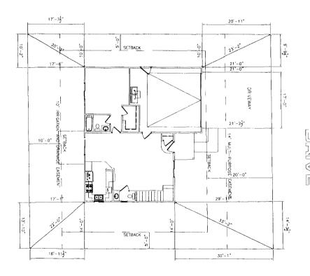
NOTE:: DIMENSION LINES ARE PULLED FROM EDGE OF BRICK LEDGE. IF NO BRICK LEDGE EXISTS, DIMENSIONS WILL BE FROM EDGE OF FOUNDATION.
