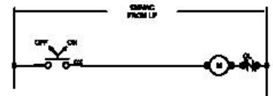
IRRIGATION PUMP STARTER SCHEMATIC (NEW STARTER FOR THIS EXISTING PUMP SHALL BE PROVIDED)
