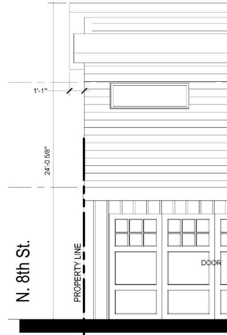
3 Roof Overhang Garage - N. 8th St. SCALE: 1/4" = 1'-0"
