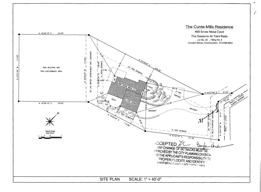
AX. NATURAL ELEVATION - DOWNSPOUT HAIN LEVEL F.F.E. 4852 SWALE W/ NATIVE ROCK ) TO PREVENT EROSION / (TYP. ALL DOWNSPOUTS) / 100 4850 4848 DECK F.F.E. OWNSPOL WASH SWALES SHALL BE AT LEAST 2' WIDE WITH A 6" DEPRESSION. ROCK SHALL BE PLACED ON A WASH WEED OR EROSION CONTROL FABRIC. fick Dom's CITY OF GJ. 8-31-10
