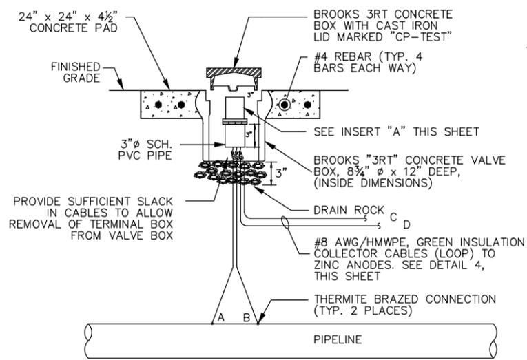
1 FLUSH MOUNTED ANODE TEST STATION
