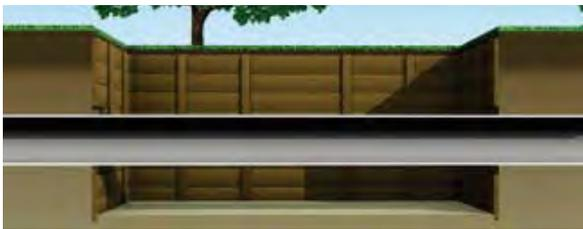
In order to uncover the old pipe, the excavation enclosure needs to be built with a sheeting or a slope.
