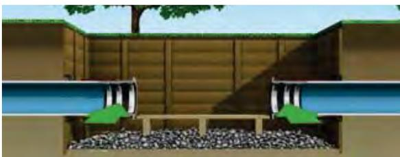
The SAERTEX-LINER® Pressure / SAERTEX-LINER® H<sub>2</sub>O shall be connected with liner end seals to the flanges.
