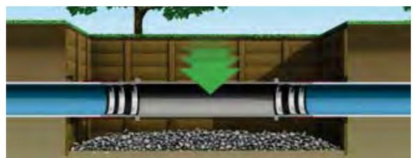
The network will be coupled to the flanged pipe section and sealed.
