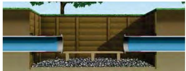
The SAERTEX-LINER® Pressure / SAERTEX-LINER® H<sub>2</sub>O will be installed and cut back.
