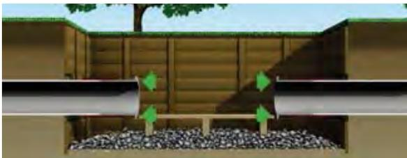
Flange adapters (Option A) or, as shown here, welded Flanges (Option B) are attached to the old pipe.
