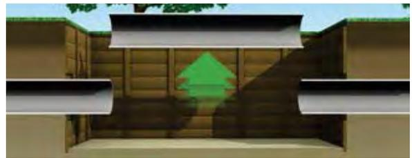
The old pipe must be cut open and the intermediate piece has to be removed.
