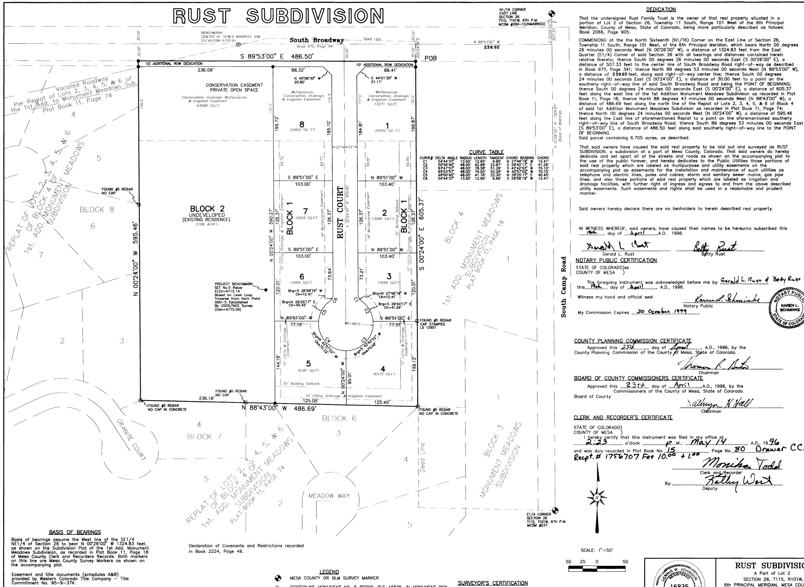
Note: Existing property corners which were recovered during this survey which were within 0.25 feet  $\pm$  of the calculated position were accepted as being "in position".
