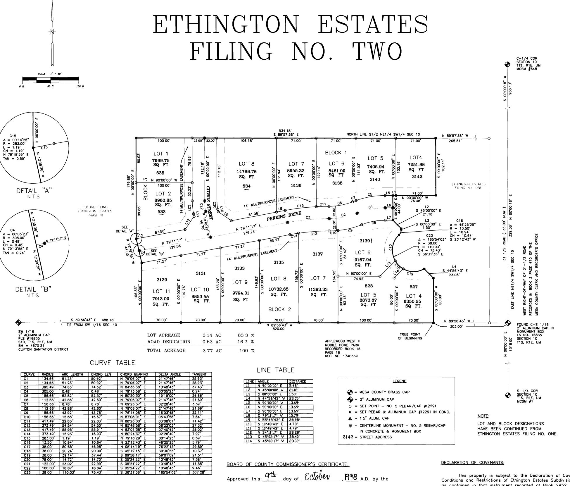
Basis of Bearings is the East line of the NE1/4, SW1/4 of Section 10, T1S, R1E, Ute Meridian, Mesa County, Colorado which bears N00°00'18"E a distance of 1317.51 feet — Ethington Estates Filing No. One.
