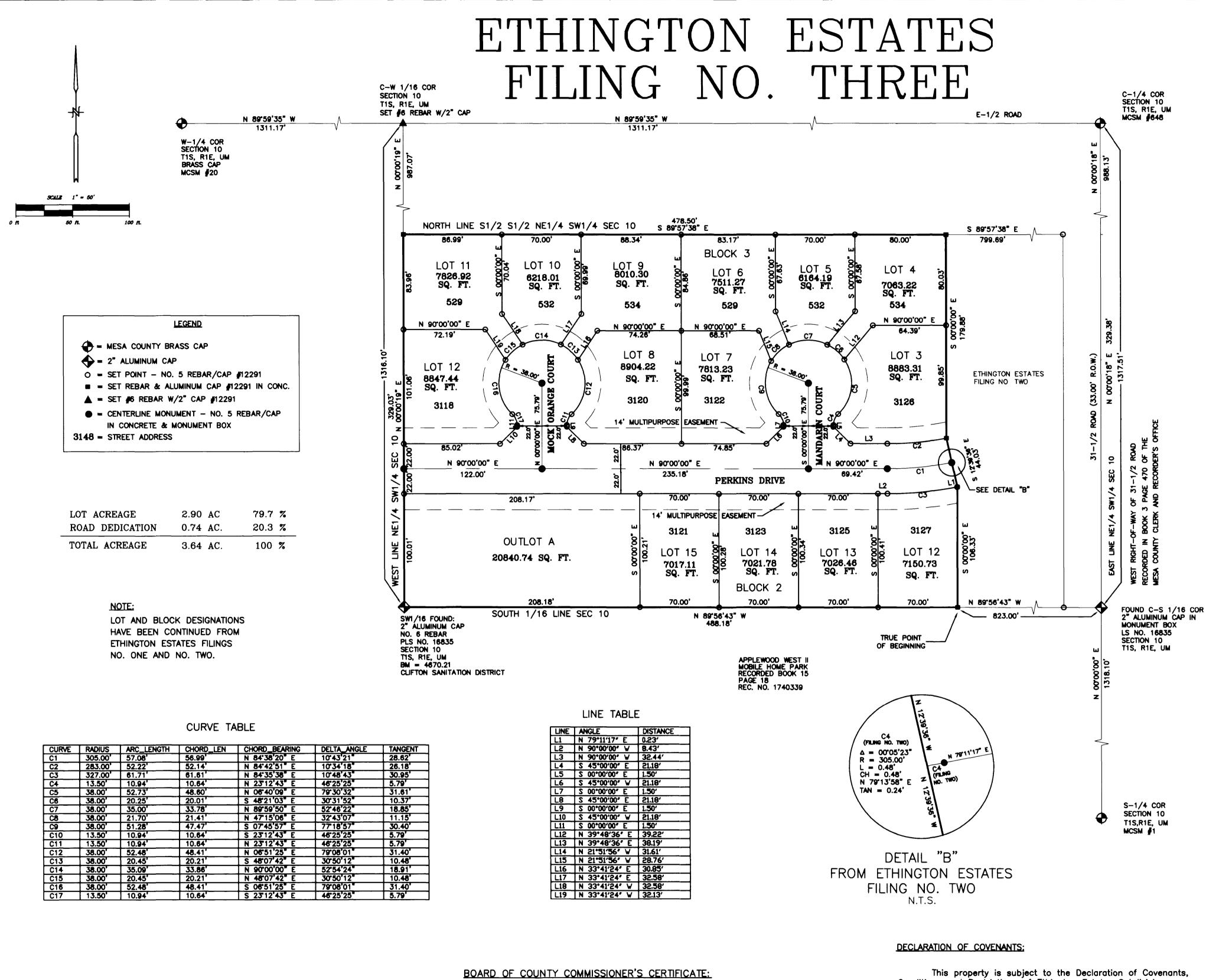
Basis of Bearings is the East line of the NE1/4, SW1/4 of Section 10, T1S, R1E, Ute Meridian, Mesa County, Colorado which bears N00°00'18"E a distance of 1317.51 feet — Ethington Estates Filing No. One.
