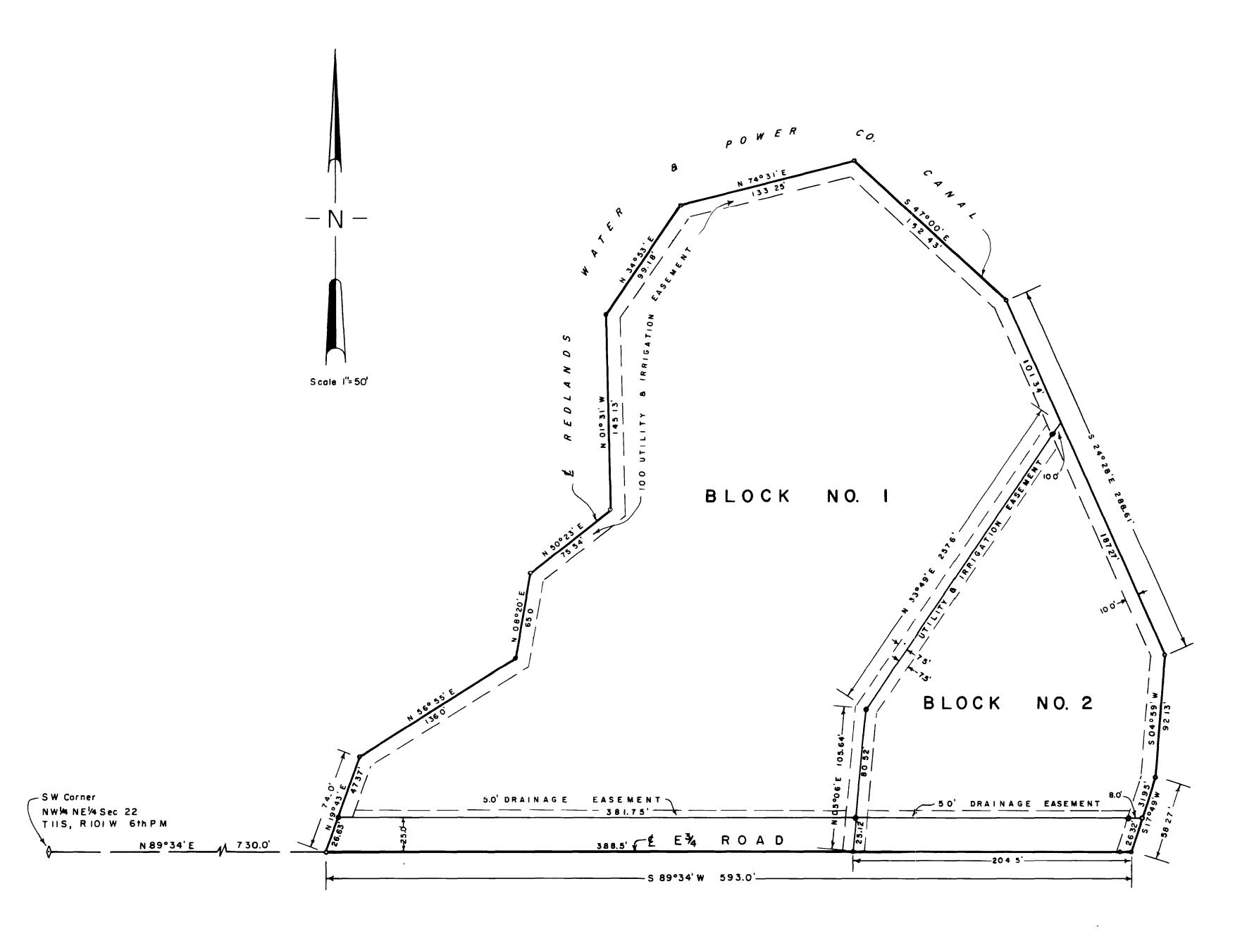
LEGEND Permanent corners set in concrete \_\_\_\_ Steel Pins
