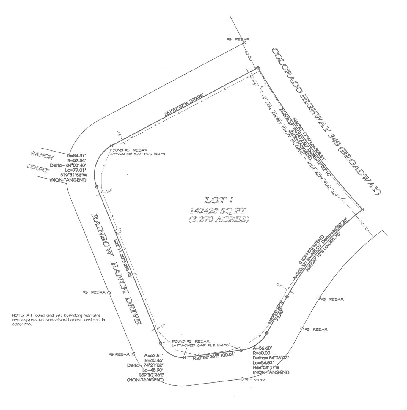
NOTE: Boundary dimensions differ from the record as follows: Found corners were accepted as original. Highway 340 right-of-way established by fitting deed descriptions to found R.O.W. monuments. New corner positions have been established by distributing errors proportionately between found corners and right-of-way. Rainbow Ranch Drive has been allowed its nominal fifty foot right-of-way based on found corners across the street. See Basis of Bearings Statement for further explanation.
