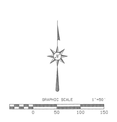
BASIS OF BEARINGS STATEMENT: Bearings are based on grid north of the Mesa County Local Coordinate System, locally determined by GPS observations on the found #5 rebars on the south line of Lot I. The measured bearing of this line is N820°58'26"E.
