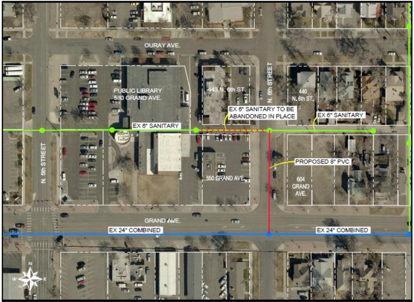
Proposed Sewer Realignment
